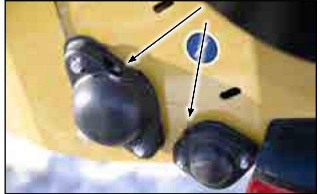
Fig 40 - Bearing grease zerks
