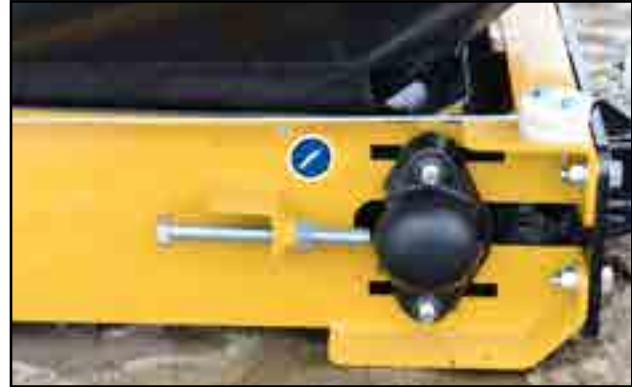
Fig 37 - Hopper roller bearing
