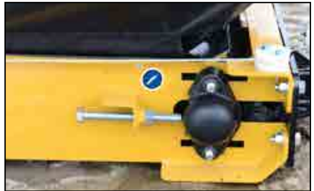
Fig 48 - Roller bearing mounts and anchor bolts
