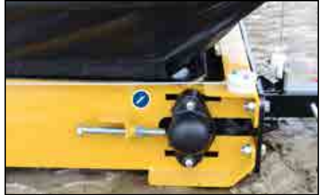
Fig 50 - Tail roller bearing housing
