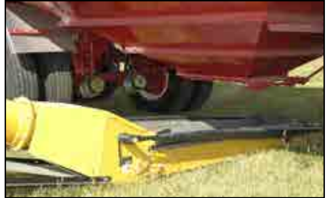
Fig 18 - Conveyor under truck
