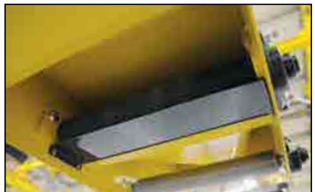
Fig 54 - Containment plate in place
