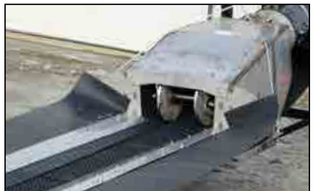
Fig 12 - Railcar hopper with hold-down wheels
