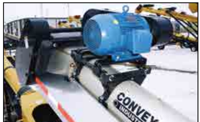
Fig 61 - Electric motor, speed reduction drive
