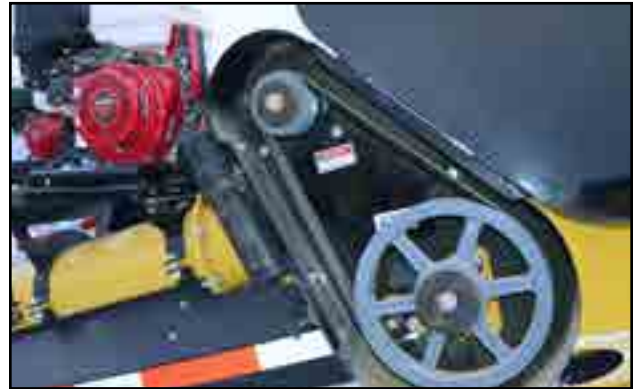
Fig 58 - Countershaft to drive roller V-belt
